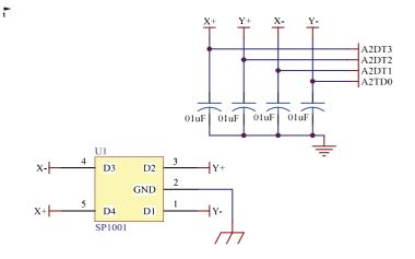
Another area of concern in terms of ESD protection are any high speed signal connectors. An ESD event can easily effect the communication signals. The use of TVS devices and ferrite beads on the USB data signals have been a long known practice.
