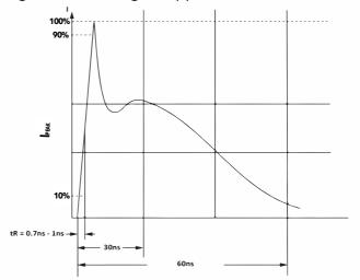
Voltage ranges from 4kV to 15kV for air discharge, and 2kV to 8 kV for contact discharge. It is this peak current that must be reduced in order to mitigate any ESDfailure. Transient voltage suppressors is commonly used in circuit design for ESD protection.
